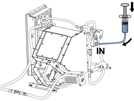
Image 2-14 Pressurize cooling circuit
